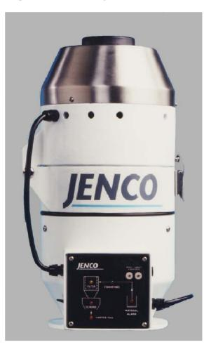
Stainless-steel / cast-aluminium construction, comprising hopper unit with material inlet, self-operating flap outlet, level- switch and replaceable dust filter. All models have automatic, pulse-jet filter- purge.
